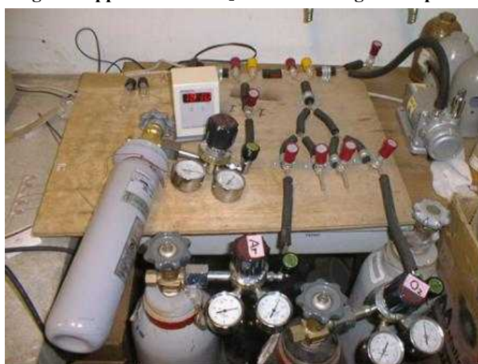
Fig 11: Gas mixing apparatus for ^{15}N_2 fixation studies
