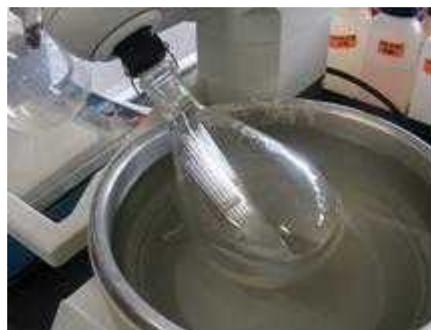
Fig. 14: Evaporation of water in Kjeldahl digested solution in Pyrex glass tubes by round bottom flask with short neck
