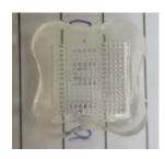
Figure 7. Hydrogel-based media cell culture from carrageenan-PVA-PEG
