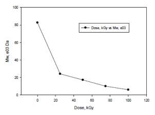
Figure 1; Effect of absorbed dose on Mw of carrageenan. Measurement was done using SEC-MALLS at 40°C of column temperature.
