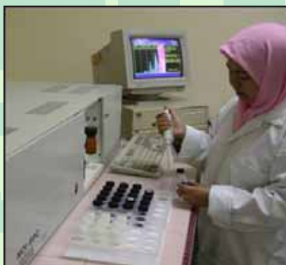
Analysis of N-15 using the emission spectrometer at MINT
