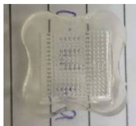
Figure 7. Hydrogel-based media cell culture from carrageenan-PVA-PEG
