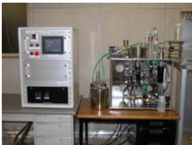
Photo 1 Automatic loading machine for Mo-99 adsorbed PZC installed at the hot laboratory of BATAN
