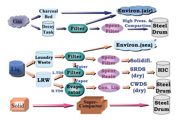
Fig. 3.5-2 Radioactive Waste Treatment Process Flow
