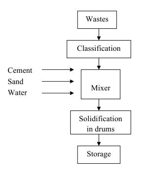
Figure 3.9-5 Flow-sheet of cement solidification
