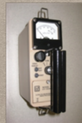
Model 9-4 Ion Chamber
